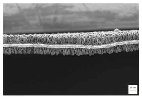
The nano-porosity of the low-density layer of silicon on each nanowire and the micro-porosity between the wires in our technology allows the silicon to expand at nano- and micro- meter levels when the anode is charged, with little to no damage to the nanowires and to the anode.
