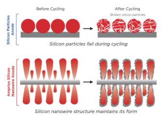
Our nanowire structure also enables ions and electrons to travel in a straight path between and through the nanowires. In contrast, a particle structure results in ions and electrons traveling in a nonlinear, tortuous path.
